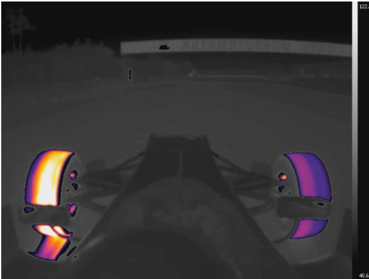
Image #2: Figure 2: Heat generated by "weaving" and braking
