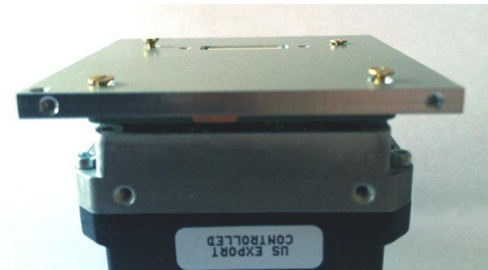
Tighten the screws carefully and make sure that the back plate does not cant. If it cants, loose the screws a little and try again. Do not apply strong forces to screws.
