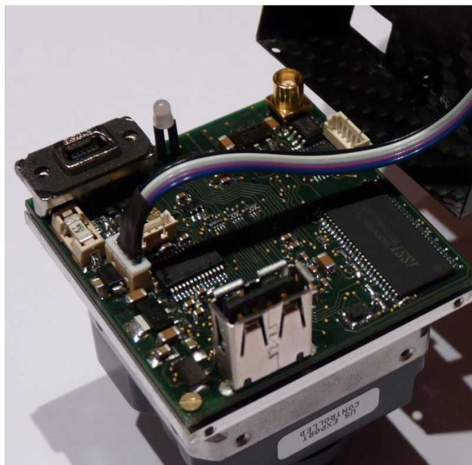
Mount the back cover and attach it with the four M1.6x3mm screws.
